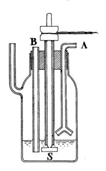
ference, which will be seen by the comparison of the present apparatus with that stated in the previous paper, is that the lower end of the tube B is dipped in the solution in the present case.
